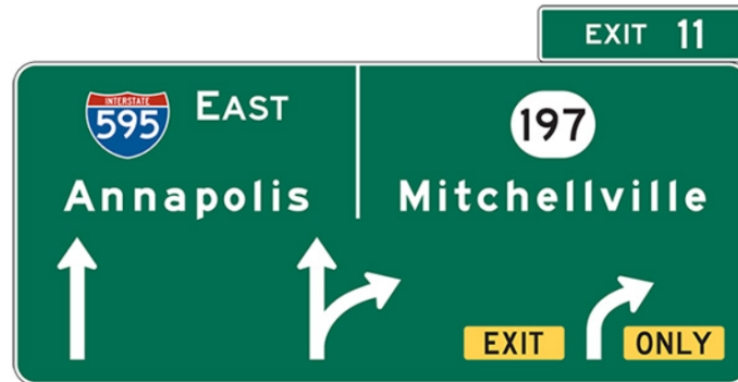
Figure 4: Diagram that demonstrates mixed-case lettering and arrow-per lane signing [30].
